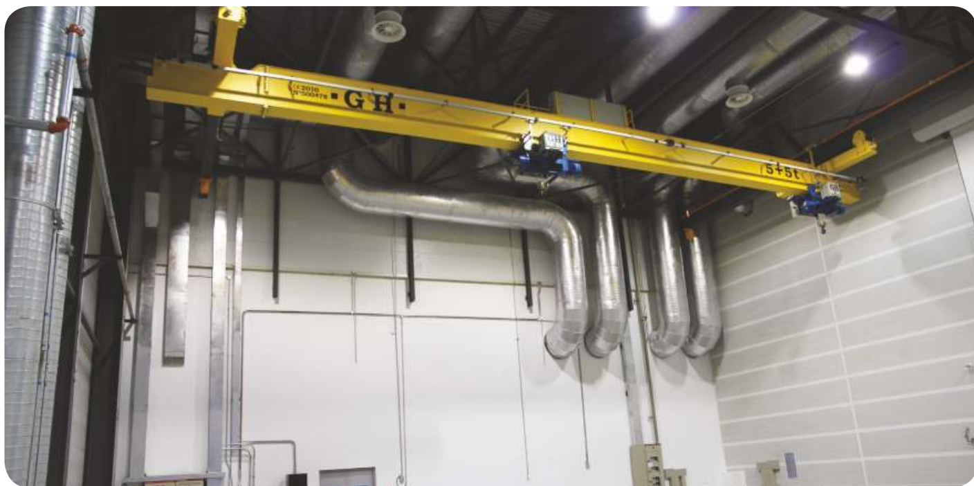
SINGLE GIRDER: CAPACITY UP TO 20+20t. 单梁起重机，额定载荷达20+20吨
