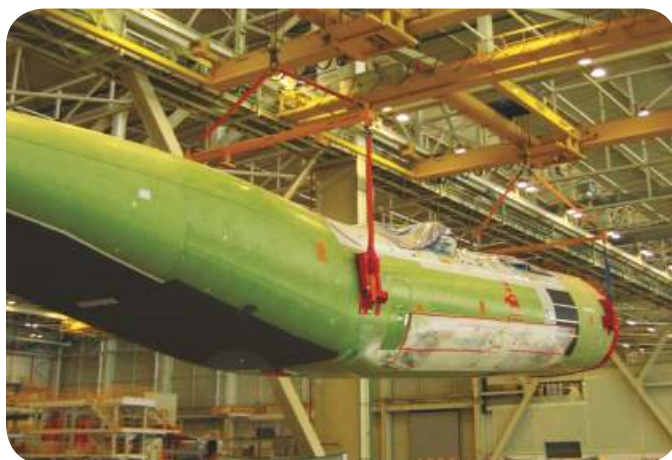
MULTIPLE POINTS UNDERSLUNG TANDEM WORKING CRANES 多吊点同步运行悬挂起重机
