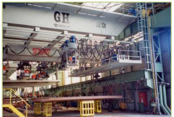
■ WELDING EQUIPMENT INSTALLED IN THE CRANE
