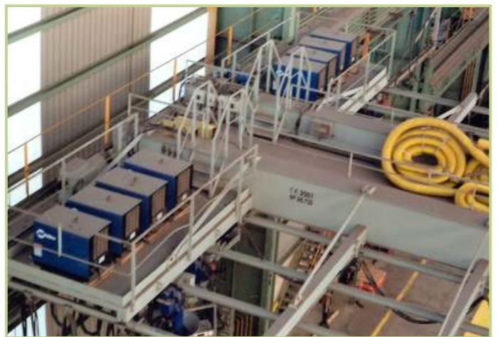
■ WELDING EQUIPMENT INSTALLED IN THE CRANE
