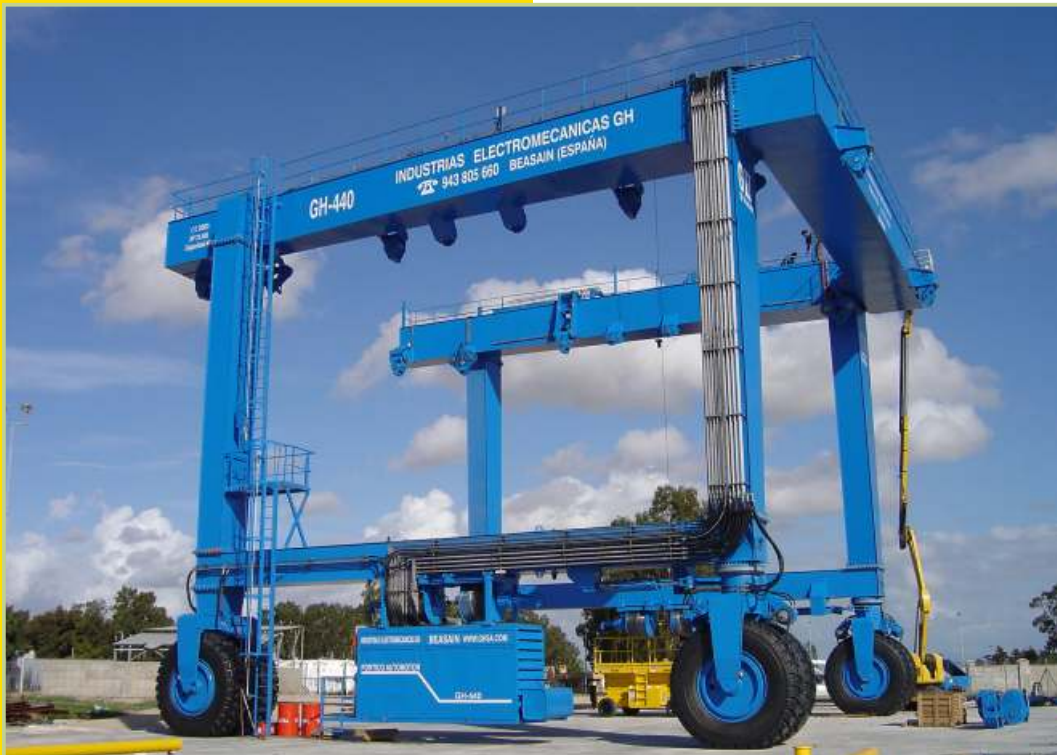
■ RUNNING VESSELS AGROUND WITH SUBMERSIBLE MOBILE BOAT HOIST
